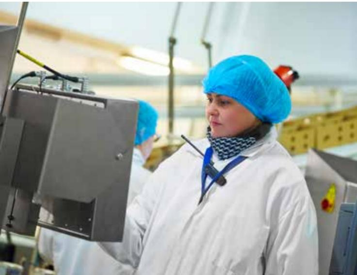
Our operator touchscreen terminals are designed with the user in mind and possess an easy-to-use, self-explanatory interface. They are versatile and robust in any production environment. Food-grade stainless steel, IP69k opto-isolated connectors, and an uninterruptible power supply are just a few of many features.
